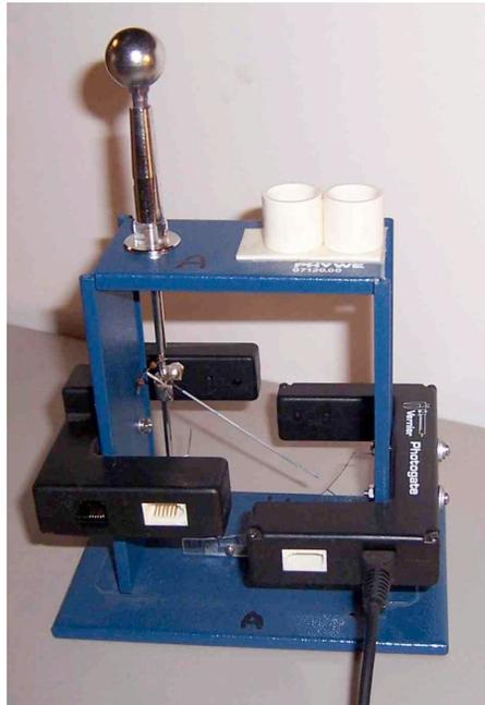
**Kolbe-type Electrostatic Monitor, with Vernier Photogates. Used for precision measurement of the time of spontaneous discharge**
