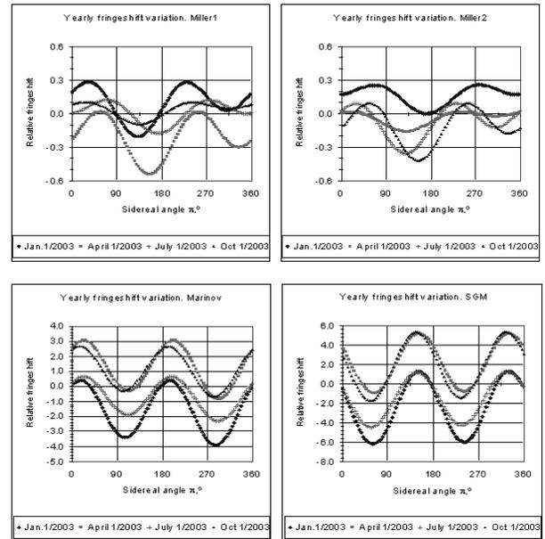
Fig. 7. Prediction of fringe-shifts at our CIF laboratory in Bogota (Colombia) for four scenarios of solar velocity, at four epochs during the year, in terms of sidereal angle  $\sigma$ , which is a proxy for sidereal time. Despite the large differences in the shape of the curves, the minima are concentrated in a small region (compare to figure 6 in terms of local civil time). The variations in position are larger for large declinations of solar velocity (Miller1, Miller2).
