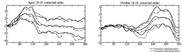
Fig. 9. Average fringe-shift curve for April (left) and October (right), corrected for H and T as measured at the eastern mirror (continuous line) and northern mirror (dashed line). The months were chosen for having a very low correlation between the temperatures at the two mirrors. The shapes of the corrected curves are similar, independently of the correction process. The one-sigma error band is shown in all cases.
