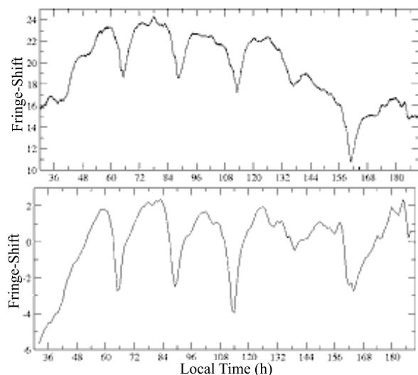
Fig. 8. Fringe-shift versus local time, as observed in the period 02 to 08 September 2003 with the green laser. Above: raw data, below: fringe-shift corrected for ambient humidity and pressure. The lower graph shows a residual curve with a periodicity similar to the original curve, with a smaller amplitude, and well defined minima.
