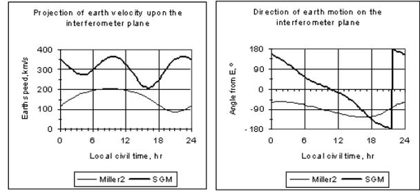
Fig. 4. Components of terrestrial motion in Cleveland (Ohio) on 8 July 1887, the first day of the MM experiment, for two scenarios of solar motion in table 3 (see text): item 4 = Miller2, and item 6 =SGM. The projection of earth motion on the plane of the interferometer depicts large diurnal variations, whose shape depends of the actual value of solar velocity. The magnitude  $V_I$  is at left, and the azimuth  $\phi$  is at the right side.
