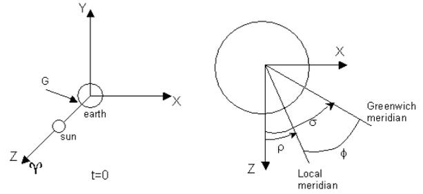
Fig. 1. Equatorial system of coordinates attached to absolute space. The Z-axis points towards the first point of Aries, which is a fixed point in space, on the date of the vernal equinox. At left, the earth as seen from the celestial north ernpole. At arbitrary time t a plane containing the Greenwich meridian makes angle  $\sigma$  with the plane defined by the Y-Z axes. An observer at longitude  $\phi$  is rotated through an angle  $\rho$  relative to the Y-Z plane.
