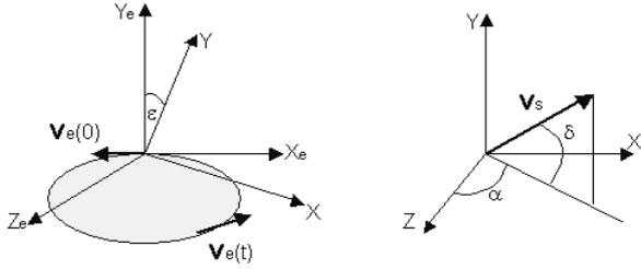
Fig. 2. The earth moves on a circular orbit with speed  $V_0$  on the plane of the ecliptic defined by the Ze-Xe axes. The equatorial system of coordinates XYZ is rotated through an angle  $\varepsilon$  with respect to the ecliptic; the directions of the Z and Ze axes coincide. At left, solar velocity  $\mathbf{V}_s$  in spherical coordinates  $(V_s, \alpha, \delta)$  in the equatorial system of coordinates.
