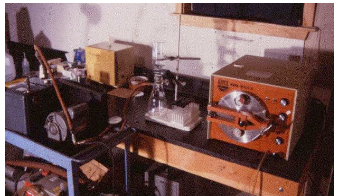
Sterilization and Filtration Equipment used for the bion experiments at OBRL.
